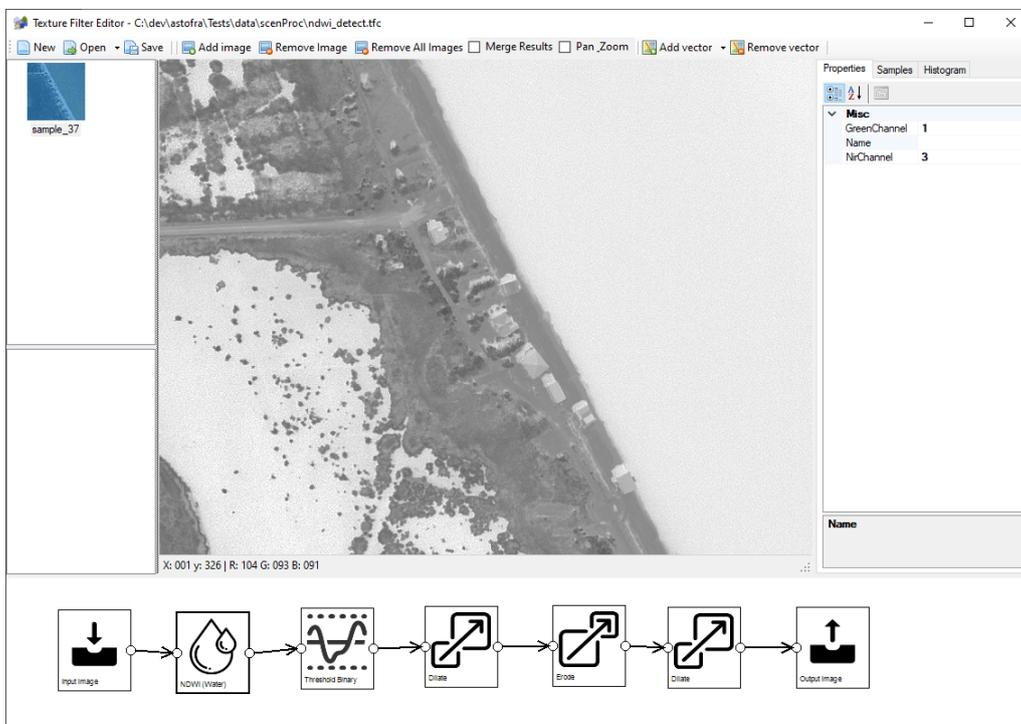
Figure 6.33: The NDWI value calculated from the input image
