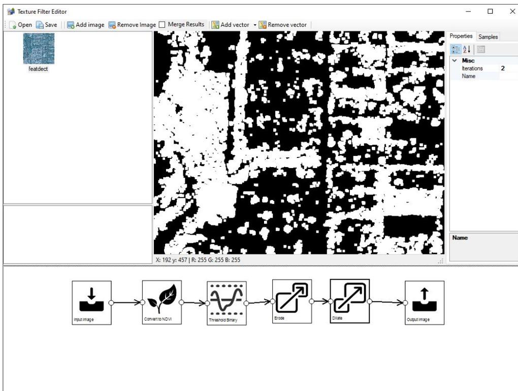
Figure 6.30: Dilating to restore the vegetation size
