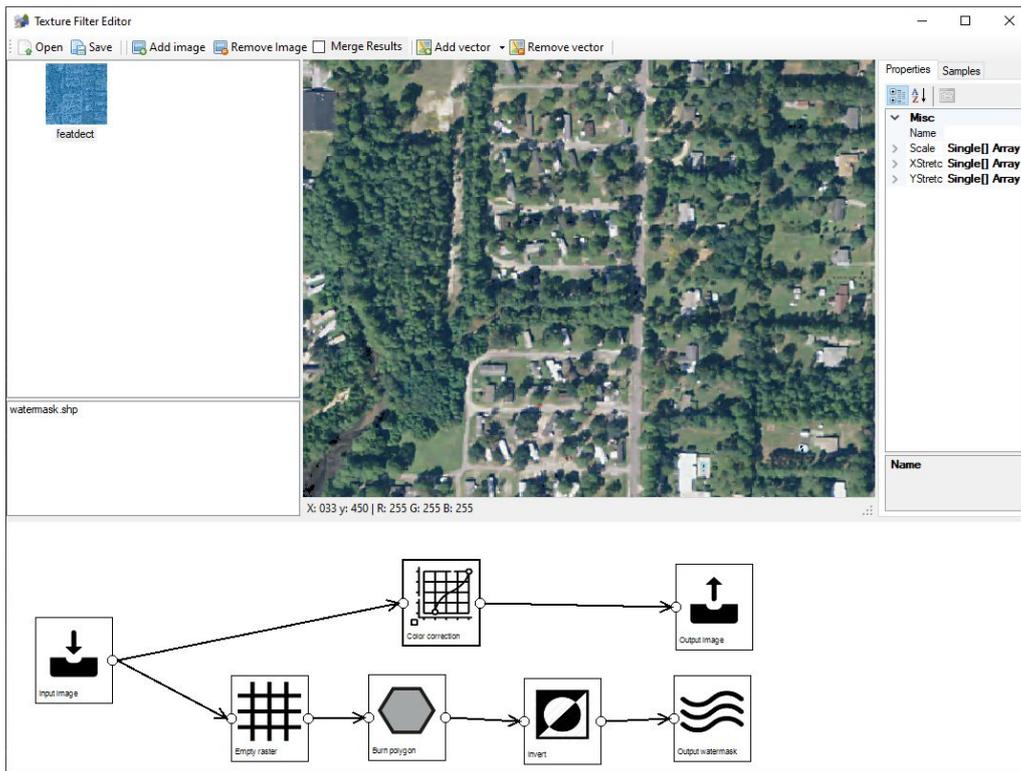
Figure 6.59: Applying color correction to the image
