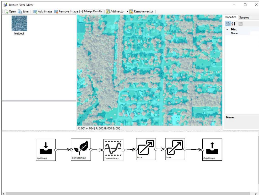
Figure 6.31: The final detection result merged with the input image
